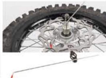
Includes a gauge to check bending of the rim and disk.
