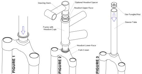
6. The star fangled nut must now be installed into the steer tube. If you don't have the set tool, we recommend dealer installation of this part. (See Figure #3)
