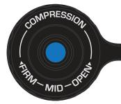
As you turn the dial clockwise, you are adding compression damping or slowing the forks compression stroke. Position two, located at roughly 3 o'clock, provides a moderately damped setting ideal for frequently changing conditions or general riding.
